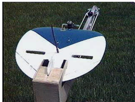
Figure 7. MLB MicroDot Circular wing 35cm MAV Winner of 1998 ISSMO MAV Competition
